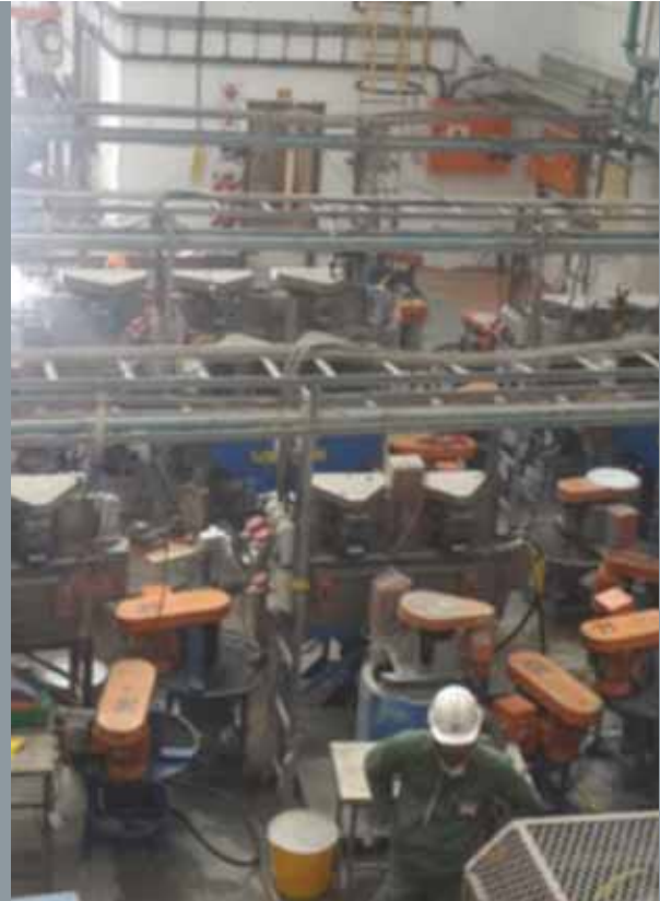
Figure 9 (b): Pilot Flotation Circuit
